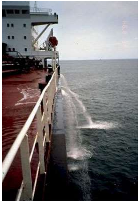
Ballast water exchange. National Ballast Water Information Clearinghouse (USA)
